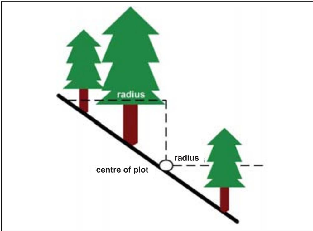
**Figure 4.2: The stepping technique of surveying slope correction on a gradient ground**
